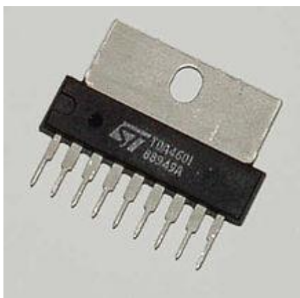
Single in-line (pin) package (SIP or SIPP)
