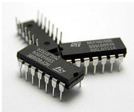
Dual in-line (pin) package (DIP, DIPP, DIL)
