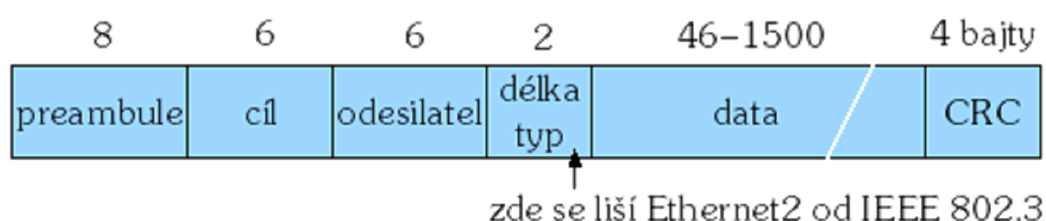
Figure 5.11-Frame format in the Ethernet network
